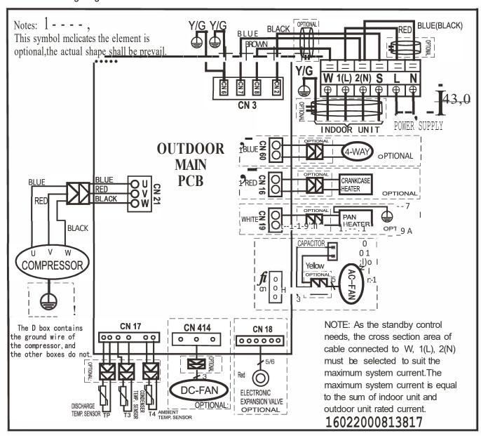
Outdoor unit printed circuit board diagram: 17122000044714, 17122000048121,17122000046453
