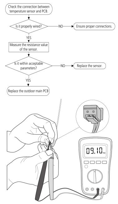
Note: For certain models, outdoor PCB could not be removed separately. In this case, the outdoor electric control box should be replaced as a whole. For certain models, outdoor unit uses combination sensor, T3,T4 and TP are the same of sensor. This picture and the value are only for reference, actual appearance and value may vary.
