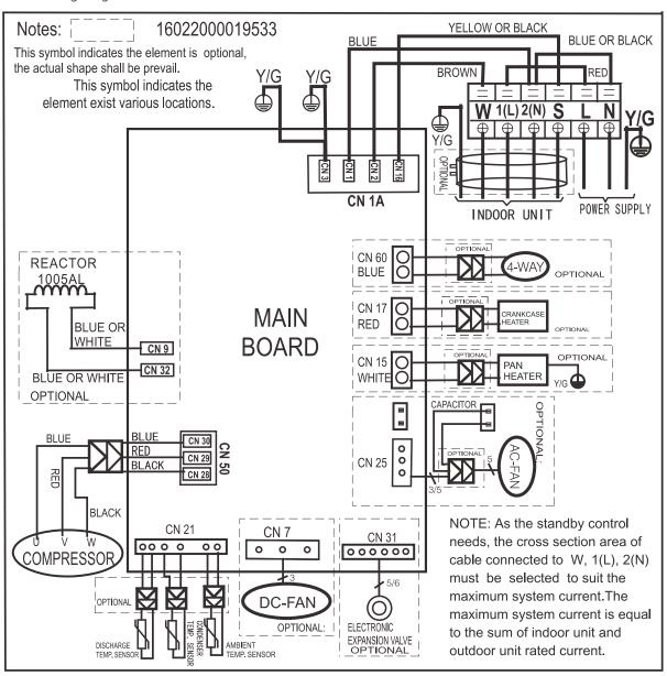
Outdoor unit wiring diagram: 16022000B13817
