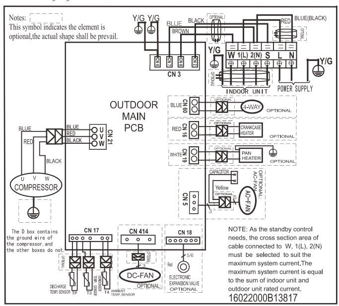
Outdoor unit printed circuit board diagram: 17122000048121,17122000046453
