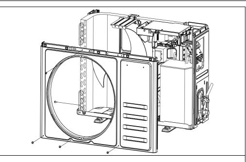
step3: Disassemble the Left and Right plate.
