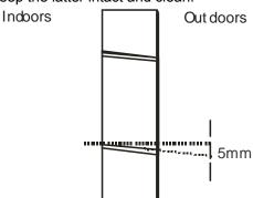
The hole must slope downwards towards the exterior. Note: Keep the drain pipe down towards the direction of the wall hole, otherwise leakage may occur.
